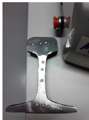
Fig. 6. Determination of chemical composition in three rail components (top, web, base)
